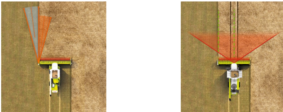
Fig. 1: Laser scanner mounted at the combine header (left) and driver's cabin (right) [3]
