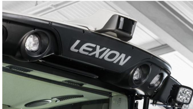
Fig. 2: CLAAS “FIELD SCANNER” sensor mounted at the cabin roof front edge [3]
