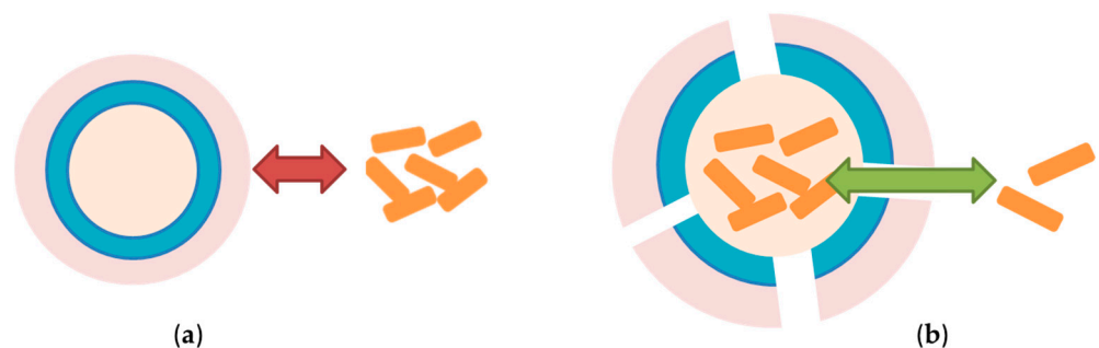
Figure 6. Schematic diagram of CM state before (a) and after PEF treatment (b), as well as respective interaction with \beta -carotene molecules.
