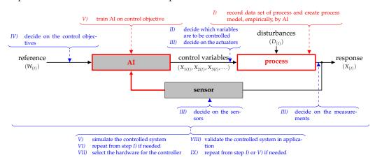
**Figure 7.** The process of AI-empowered and -based control system design, 9 steps in accordance with the corresponding block of the block diagram. Blue steps are identical to the steps of Skogestad and Postlethwaite [1]—red steps are altered; blocks with gray background are crucial for safety of the CLCS.
