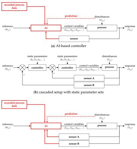
(c) simplification due to AI-based controller
