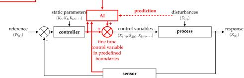
(b) AI-based controller with a limited impact on the control values
