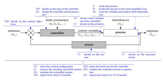
**Figure 3.** The process of control system design, first 14 steps of Skogestad and Postlethwaite [1] in accordance visualized with the corresponding blocks of the CLCS block diagram—blocks with gray background are crucial for safety of the CLCS.
