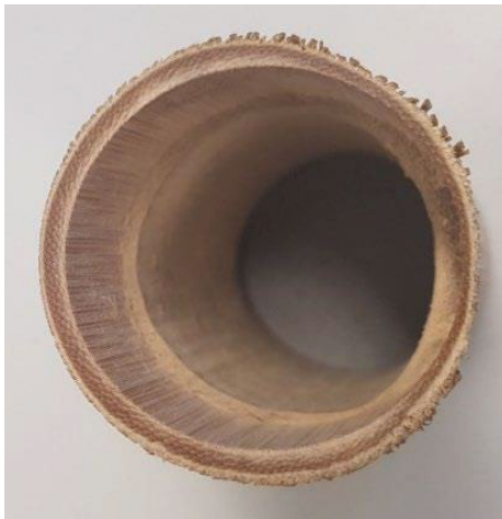
Drilled out culm
