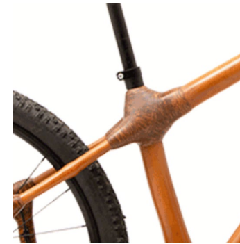
Connection wrapped with hemp ropes
