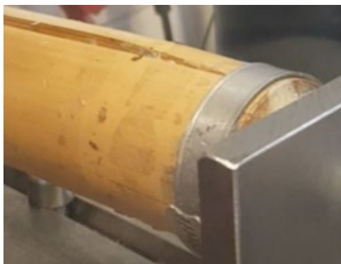
split without reinforcement
