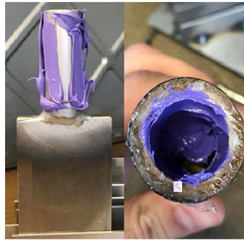
Connector & culm wetted with adhesive
