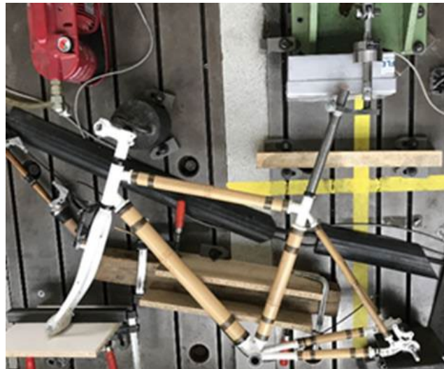
Test with a vertical force on the saddle mount
