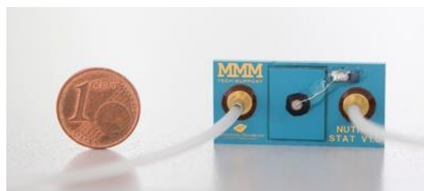
Figure 4. NUTRISTAT analysis module with ISFET measuring technology (lab-on-chip) to measure \text{NO}_3^- , \text{K}^+ and \text{H}_2\text{PO}_4^- as well as pH and electrical conductivity
