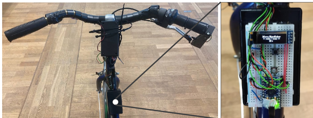
Figure A5. Cyclist’s point of view with the installed sensors and the hidden control box.
