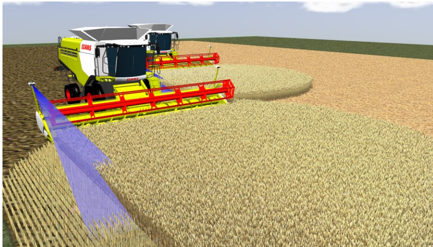
Fig. 6: LiDAR-sensor-based edge detection with 3D-surface model of crop plants
